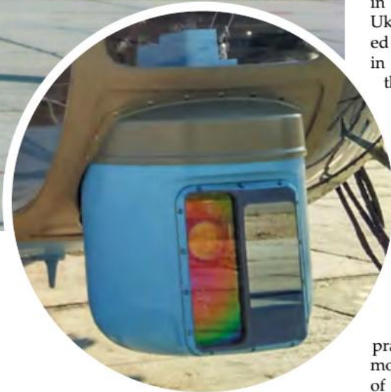
Optronic sensor turret PM LKT Spectrum can identify a tank-size target at ranges no less than 8,000 m in day-time and beyond 6,000 m at night. With laser-assisted guidance, the missile aiming range is between 50 and 7,500 m, with a CEP not exceeding 0.8 m whatever the aiming distance is.
