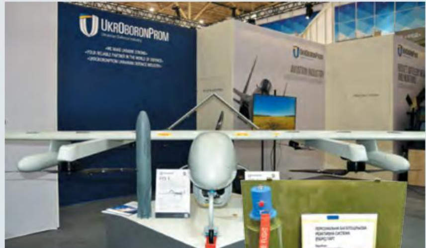
This new evolution of the PD-1 UAV platform carries two loitering munitions, each armed with a 3 kg warhead and designed to be deployable from hardpoints on each of the wings.
